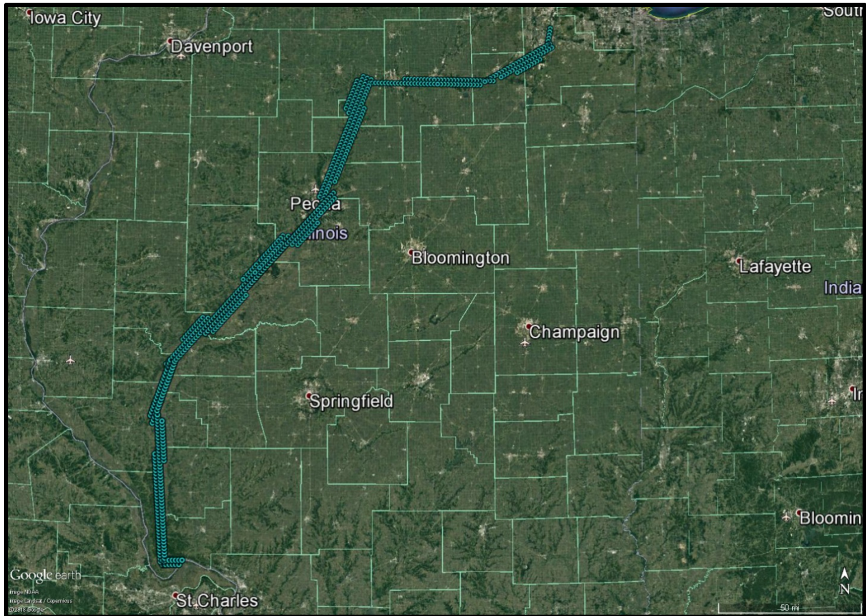
Figure 1. Lock and dam closure flight plan for the Alton Pool to Brandon Pool of the Illinois River. Note that only the main channel and adjacent backwater imagery will be collected.
