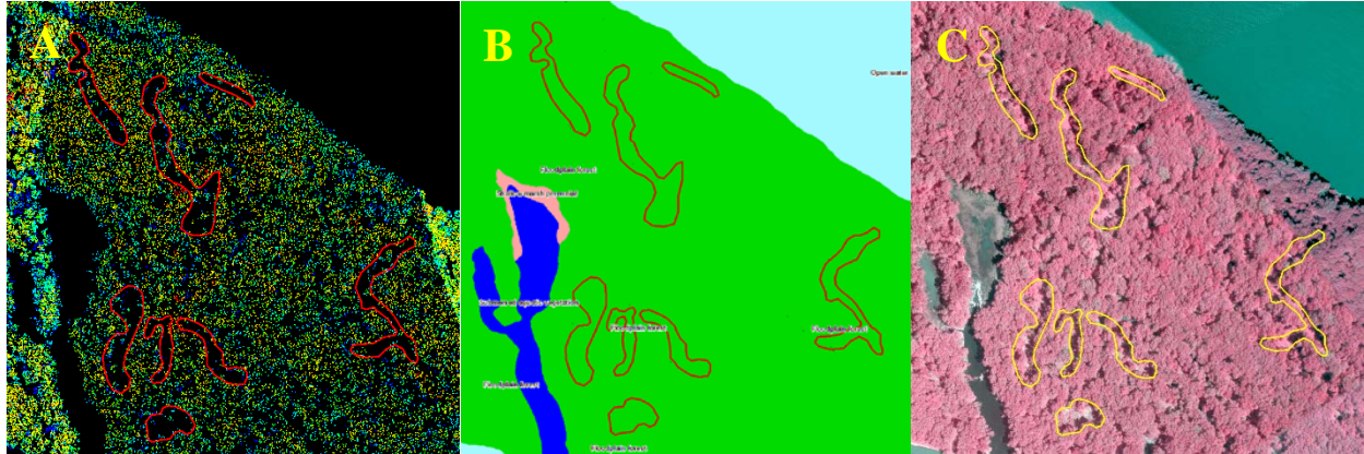
Figure 1: Tile A showing the lidar point cloud along the eastern shore of Railroad Island in Pool 13 with gaps delineated, Tile B showing how these gaps align with the existing 2010 systemic vegetation layer, and Tile C showing these same gaps in the 2010 systemic CIR imagery set.
