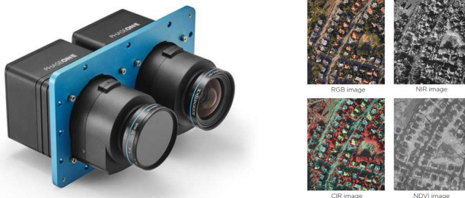
Figure 1. The 4-band Phase One RGB and Achromatic camera system with base plate and image samples.
