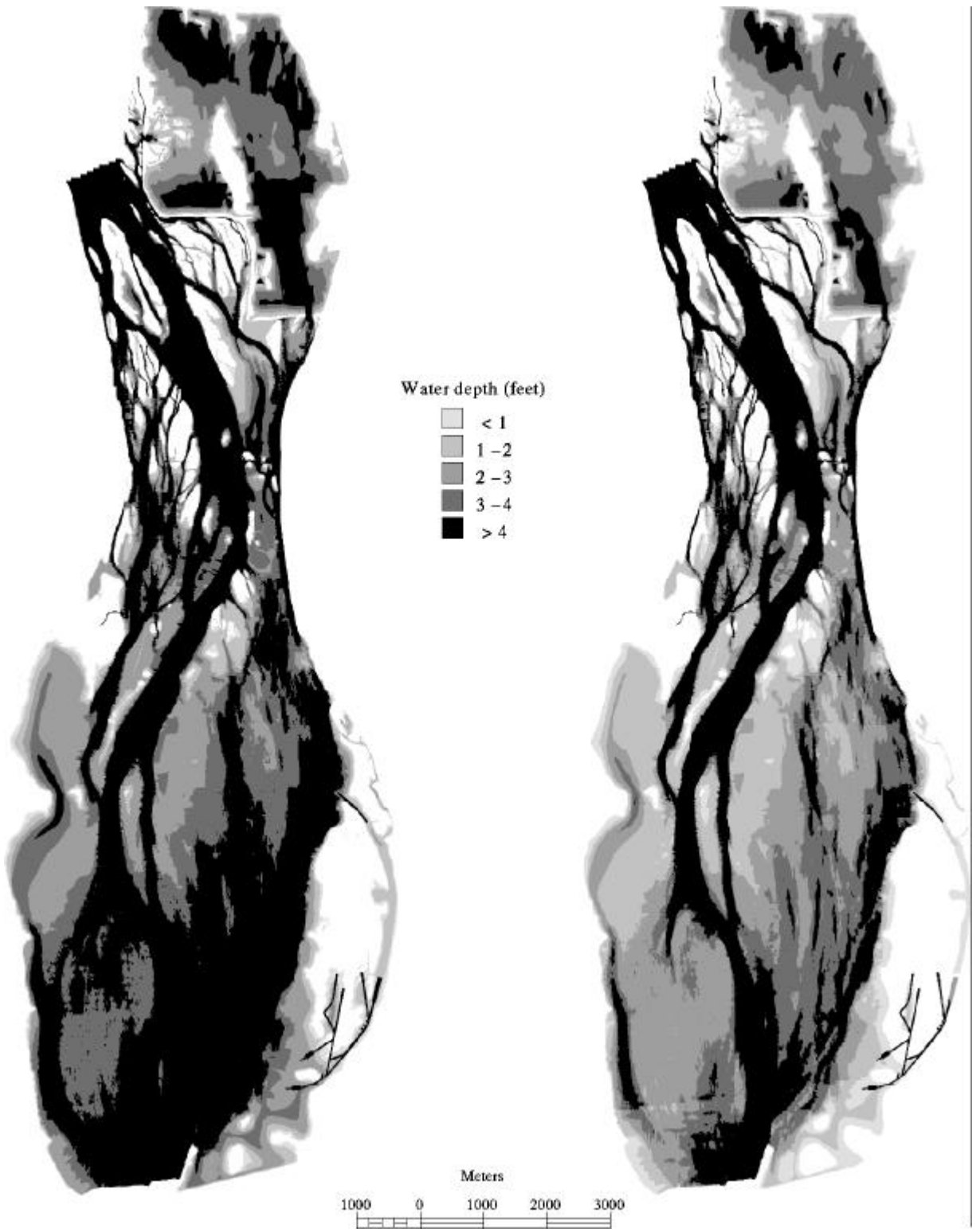
Figure 10. Maps of water depth, at 70,000 cfs, for the study area of Pool 13 when water levels at the dam are held at 583 feet (left) and 581 feet (right) above sea level.
